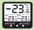
Make sure that MIN and MAX show on the display and not alarm settings (LO and HI).
